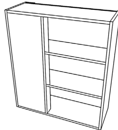
TALL STANDARD CORNER WALL UNIT with a 300 blanking panel
